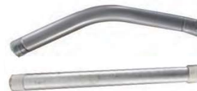
Rod: Galvanized steel with paint, M25*1.5 male thread at two ends 30/45/90/180°elbow is optional 30-50cm length IP66
